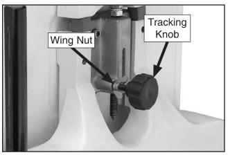
Figure 24. Tracking knob and wing nut.
